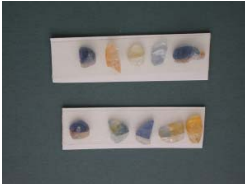
Figure 17: Samples from the Getaheta, Rantapura and Buttala area heat treated at 1800°C in air
