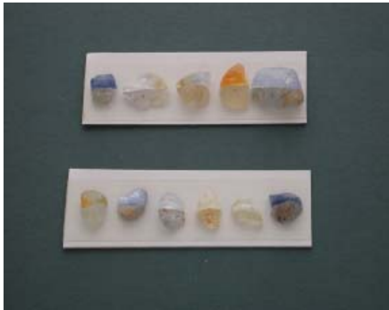
Figure 18: Samples from the Getaheta, Rantapura and Buttala area heat treated at 1800°C in air
