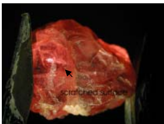
Figure 3: Surface were scratch with a mineral of hardness of 8.5
