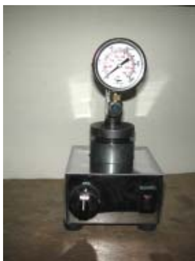
Figure 1: Equipment to fill cracks in emerald with organic substances
